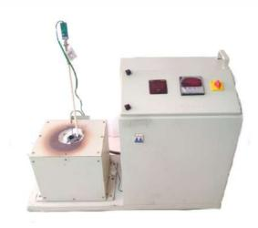
THERMOCOUPLE & RTD SENSORS TESTING BATH TEMP. RANGE: 50 TO 1100 Deg. C
